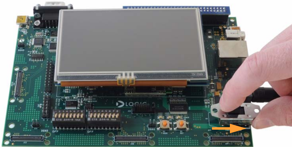
Figure 2.8 – Switch Power On
